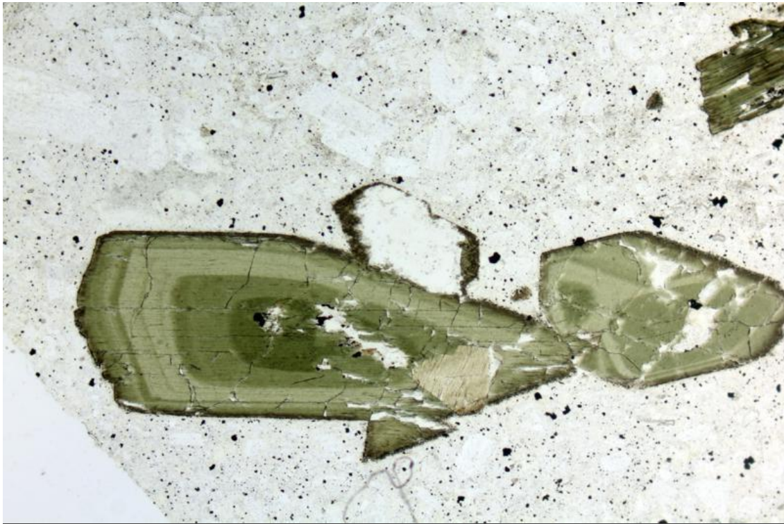
A zoned hornblende crystal in an andesite from Greece in thin section under uncrossed polarization with a petrographic microscope (field of view is 7 mm). The different colors of the zones represent different periods growth with different compositions; https://www.alexstrekeisen.it/immagini/vulc/orneblendaverde2013(2).jpg
